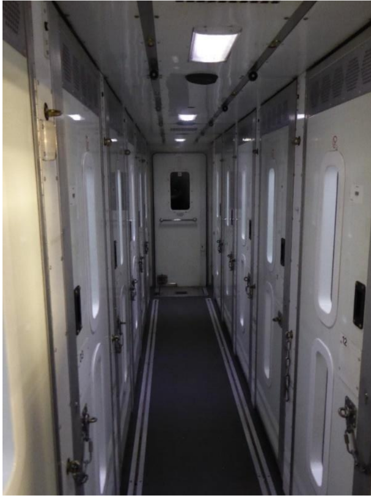
Figure 1: Inside a 12-cell prison van, showing the corridor with cell doors on either side. Each door includes a viewing window into the cell. A separation screen can be deployed at the end of the corridor to shield the final two cells from view.
